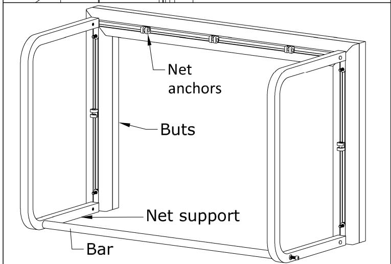
Put the hooks slat base supporting the posts and crossbars, mount the network
