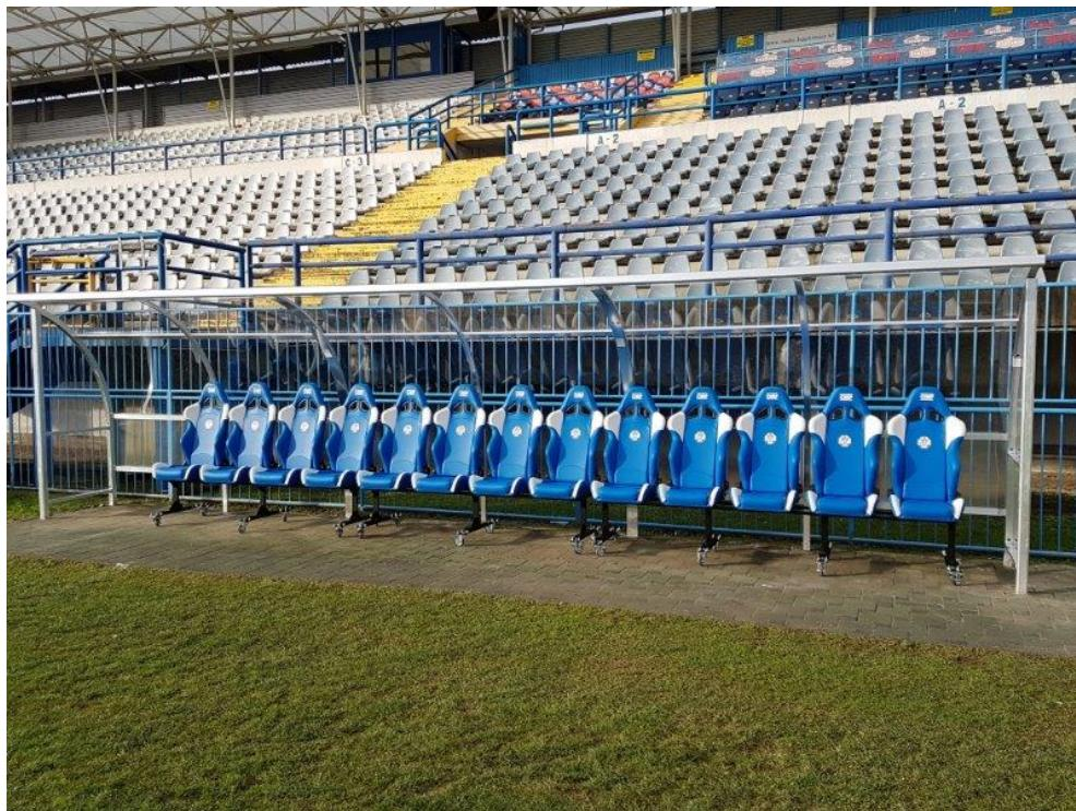
Team shelter model "Strong Plus" 5 m. long (10 seats), in aluminium, front struts construction mm. 60x70, polycarbonate panels transparent thickness mm. 3, seats in polypropylene.
