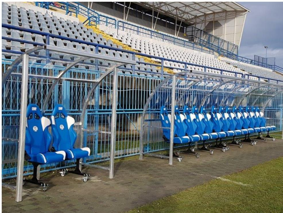
Team shelter model "Strong Plus" 6 m. long (12 seats), in aluminium, front struts construction mm. 60x70, polycarbonate panels transparent thickness mm. 3, seats in polypropylene.
