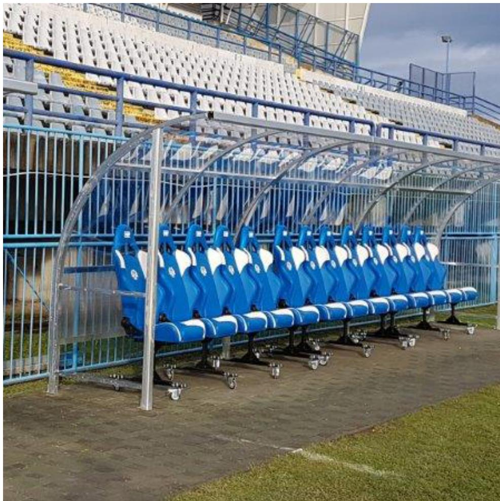
Team shelter model "Strong Plus" 4 m. long (8 seats), in aluminium, front struts construction mm. 60x70, polycarbonate panels transparent thickness mm. 3, seats in polypropylene.
